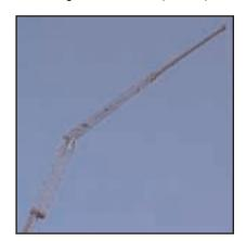
Optional 20 ft. (6.1 m) or 40 ft. (12.2 m) swingaway extension insert; Maximum tip height: 20 ft.--194 ft. (59.1 m); 40 ft.--214 ft. (65.2 m)
