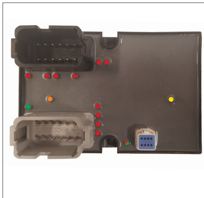
Figure 3-15: LED indicator lights (transmitter)
