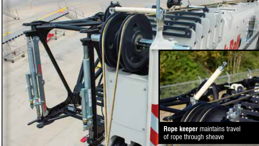
Quick reeve boom head eliminates the need to remove the bucket when it becomes necessary to change the reeving
