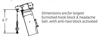
\*Drawing is to show the physical reach of the machine. Always refer to load chart to see what portions of this range are structurally and stability limited.
