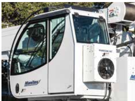
Operator cab reclines from 0° to 20° for a comfortable, clear view of the load.
