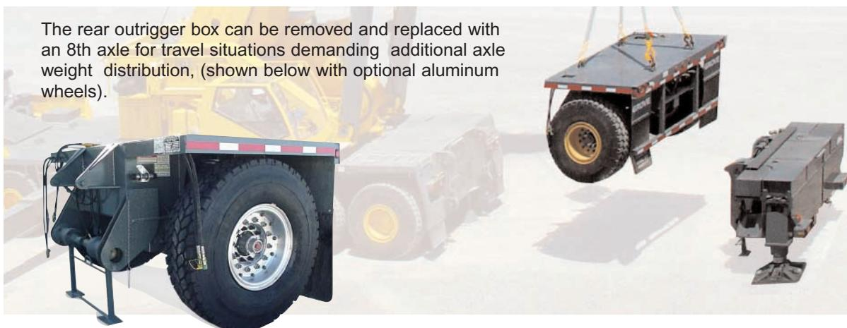
The rear outrigger box can be removed and replaced with an 8th axle for travel situations demanding additional axle weight distribution, (shown below with optional aluminum wheels).
