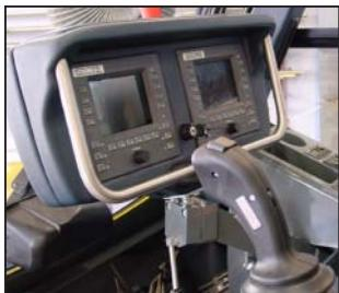
The operator's cab on the GMK7550 uses the new EKS5 LMI system and ECOS (Electronic Crane Operating System) with a combined dual screen display mounted on a tiltable swing arm.
