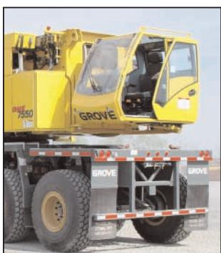
The new superstructure cab stows to the rear and swings hydraulically to the right side of the crane for operation. Stationary heating and A/C are standard.
