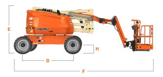
A. Platform Width 30-in / 0.76-m B. Platform Length 72-in / 1.83-m Machine Width 7-ft 8.6-in / 2.35-m Tailswing Zero 7-ft 5.3-in / 2.27-m 21-ft 6.9-in / 6.57-m
