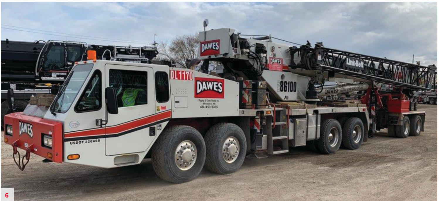
Link-Belt HTC86100, S/N N3K2-3055 2012, 100 USt, Cummins ISX11.9, 11,891 Hours, 50,820 Miles, 140' Main Boom, 35'-58' Offset Jib, Aux. Hoist, Trailer Air & Electric, 39,500# Counterweight, RCL Light Bar, A/C, 2 Axle Boom Dolly. Located in Milwaukee, WI. Unit #DL1170MLW. $479,000
