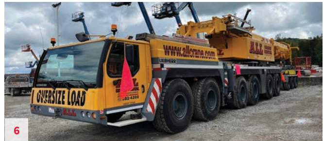
Liebherr LTM1250 6.1, S/N 070980 2013, 300 Ust, Liebherr Diesels, 7,058 Upper Hours, 3,700 Lower Hours, 58,000 Km, ZF Trans, 236' Main Boom, 40'-70' Swingaway Jib, (2) 23' Jib Inserts, Winch 2, 214,500 lbs. of Counterweight, Removable Main Boom, Removable Rear Outrigger Boxes, A/C, Boom Dolly, Located In Pittsburgh, Pa. Unit #10668. $1,600,000
