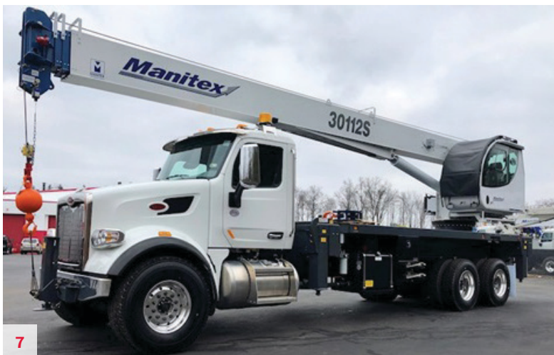
NEW Manitex 30112S 30 USt, 112' Main Boom, Jib Ready, Front Bumper Hyd Stabilizer for 360 Load Chart, Free Swing Option, A/C in Operator Cab, Out & Down Outriggers, and Extra Control Valve for an accessory. Mtd on a Peterbilt 567 Chassis, Cummins X15/500 HP, Allison 4500 Automatic Trans, 100 Gallon Fuel Tank, 20K FA, 46K Tandem, Air Disc Brakes, Zinc-Coated Frame Rails, and MUCH MORE. (Stock Photo). Unit #R2388
