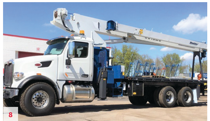
NEW Manitex 30102C 30 USt, 102' Main Boom, 26'-46' Jib, Front Bumper Hyd Stabilizer for 360 Load Chart, Out & Down Outriggers, Oil Cooler, and Extra Control Valve for an accessory. Mtd on a Peterbilt 567 MX-13 Engine 510HP, Eaton 13-spd Ultrashift plus Transmission, 20K FA, 46K Tandem, Air Disc Brakes, 80 Gallon Fuel Tank, and MUCH MORE. (Stock Photo). Unit #R2297
