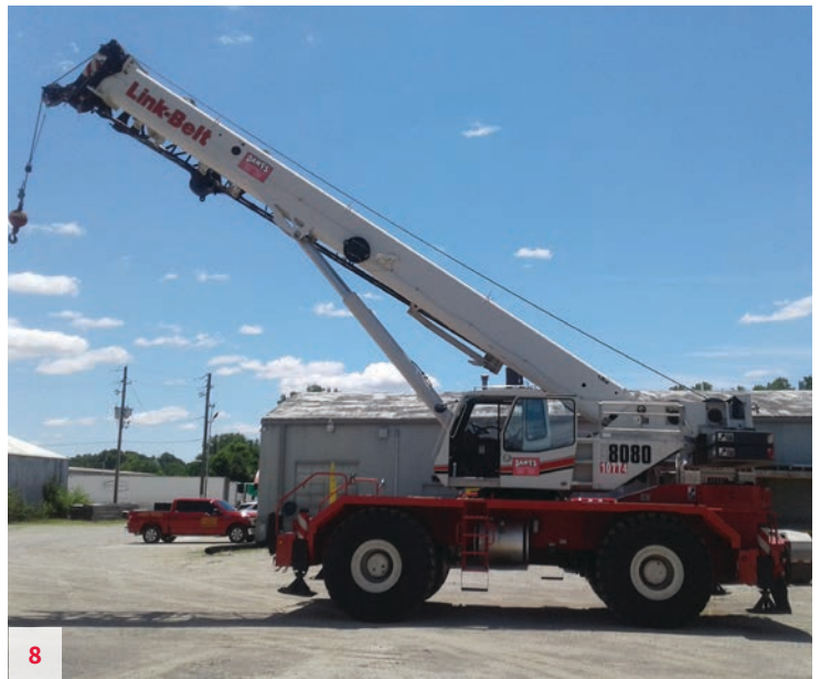
Link-Belt RTC-8080 II, S/N S4K3-3435 2013, 80 USt, Cummins Diesel (6,800 Hours), 127' Main Boom, 10'-38'-64' Offset Jib, Aux. Hoist, 19,200# Counterweight, RCL Bar Graph, A/C, Joystick Control, Block and Ball. Located in Hammond, IN. Unit #10774. $327,000
