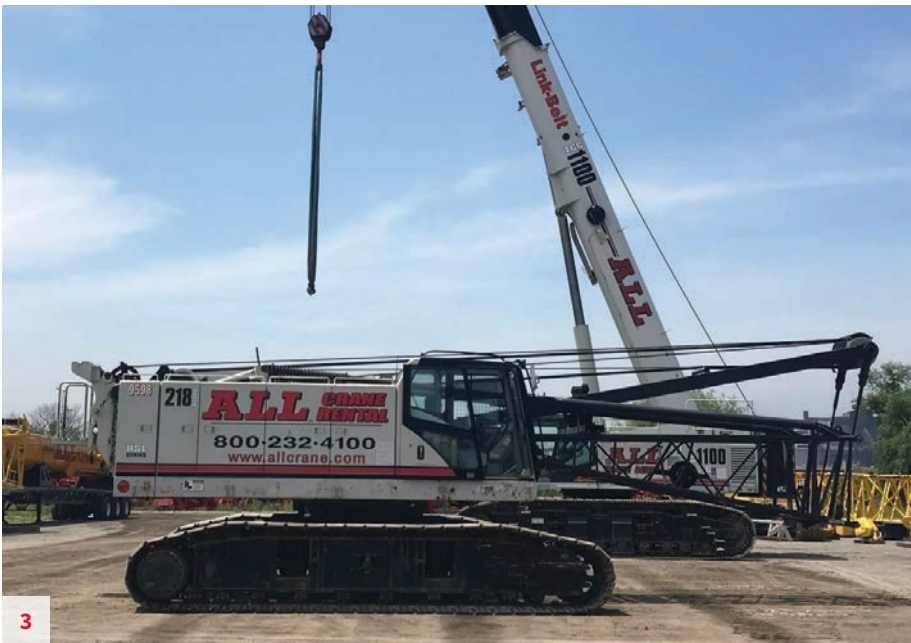
Link-Belt LS218HSL, S/N N6J7-9021 2007, 110 USt, Isuzu 6HK1 Diesel Tier III (19,740 Hours), 140' Main Boom, 3rd Drum, Free Fall, Rebuilt Tracks in 2018. Newer Paint. Located in Hamilton, Ontario. Unit #9598. $297,000
