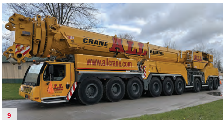
Liebherr LTM 1750-9.1 - S/N 096248 , 2019, 900 USt, Liebherr Diesels, 3,311 Upper Hours, 1,541 Lower Hours, 17,725 Miles, 171' Main Boom, 299' Luffing Jib, Y-type Guyed, Blocks and Ball. Located in Fort Wayne, IN. Unit #11504 Call for price
