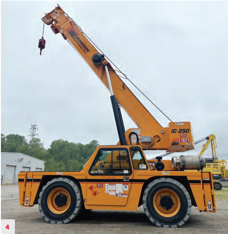
Broderick IC-250-3E - S/N 77438250 , 2023, 18 USt, GM5.7L V8 EPA Tier II LPG Fuel Only, 489 Hours, 50'1" Main Boom, 20' Offset Jib, Four Wheel Steer and 4 Wheel Drive, High Traction Tread Non-Marking Tires, Rear Pintle Hook, All Weather Cab (Heater, Defroster, & Wiper), Strobe Light, Boom Work Lights, Rated Capacity Limiter, Drum Rotation Indicator, 4 Part Block and Ball. Located in Pittsburgh, PA. Unit #11821 $317,000
