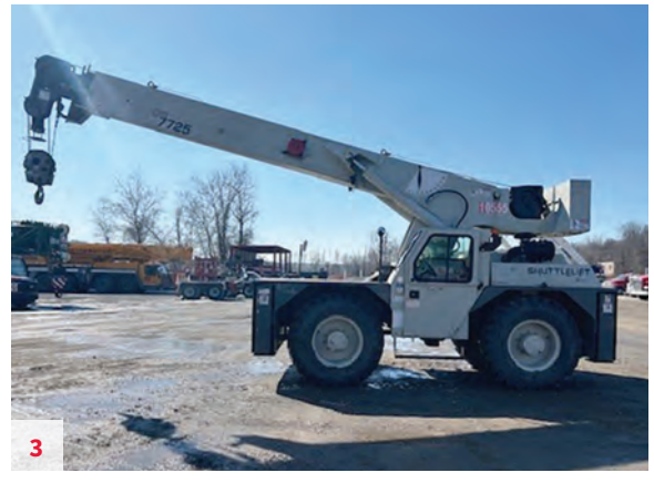
Shuttlelift 7725 – S/N 321884 , 2012, 25 USt, Cummins QSB4.5, 7,680 Hours, 71' Main Boom, 17' Jib, 4x4, Catalytic Converter, Aux. Lighting Package, Enclosed Cab Package, Outrigger Monitoring System, LMI, Block and Ball. Located in Pittsburgh, PA. Unit #10555 $177,000
