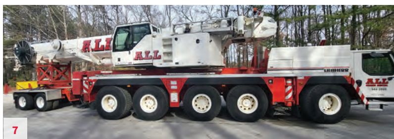
Liebherr LTM 1160-5.1 - S/N 067563 , 2013, 190 USt, Liebherr Diesels 8,862 Upper Hours, 2,389 Lower Hours, 45,279 Miles, 203' Main Boom, 40'-72' Hydraulic Offset Swingaway Jib, 23' Intermediate Section, 23' Extension of Telescopic Boom, Rooster Sheave, Second Hoist, Second Boom Head Top Sheave, 20.5 R25 Tires, Supporting Base Detection, A/C in Upper and Lower Cabs, 102,300 lbs. Total of Counterweight, 2 Axle Boom Dolly, Block and Ball. Located in Atlanta, GA. Unit #10687 $965,000
