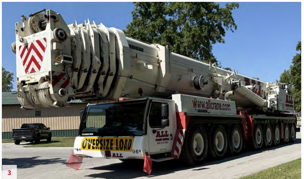
Liebherr LTM1500 8.1 - S/N 095255 , 2012, 600 USt, Liebherr Tier 3, 9,411 Upper Hours, 3,202 Lower Hours, 49,496 KM, 276' Main Boom, 298' Luffing Jib, Y-Guy, 2 Winches, 20.5 R25 Tires, A/C, 8 Counterweight slabs each with 16,500, Removable Telescopic Boom, Additional Fuel Tank, Telma Brake, Working Lights, Liccon, Special Design and Assembly for Nelson Boom Launching Lugs, Blocks and Ball. Located in Hammond, IN. Unit #10518 $1,783,000
