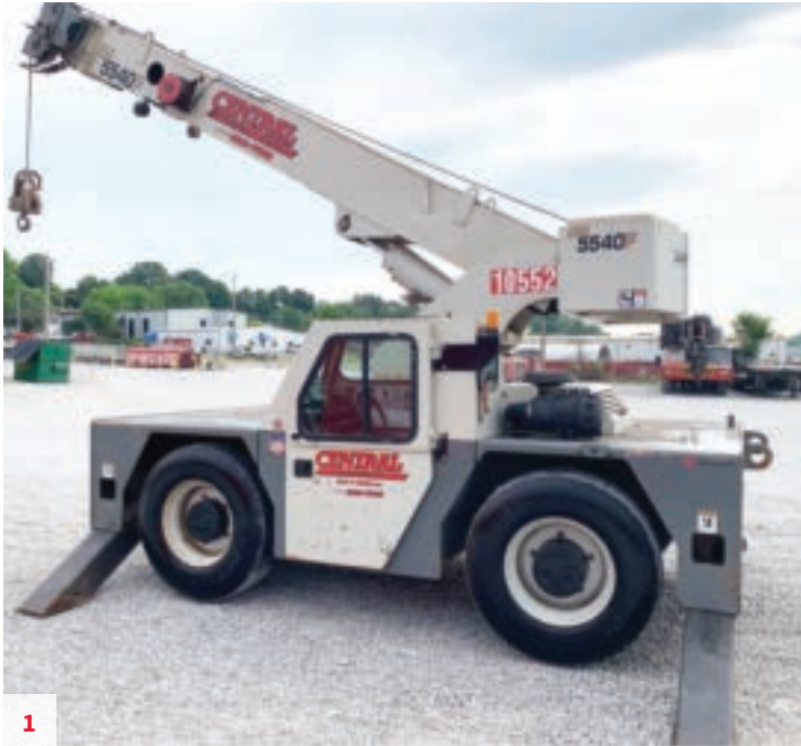
Shuttlelift 5540F - S/N 321881 , 2012, 15 USt, Cummins QSB3.3 (3,678 Hours), 41' Main Boom, 15' Offsettable Jib, 2 Wheel Drive, 4 Wheel Steer, Enclosed Cab, Lifting and Tie Down Lugs, Load Indicator, Strobe Light, Headlight and Taillight Grilles, Cab Dome Light. Located in Knoxville, TN. Unit #10552 $90,000
