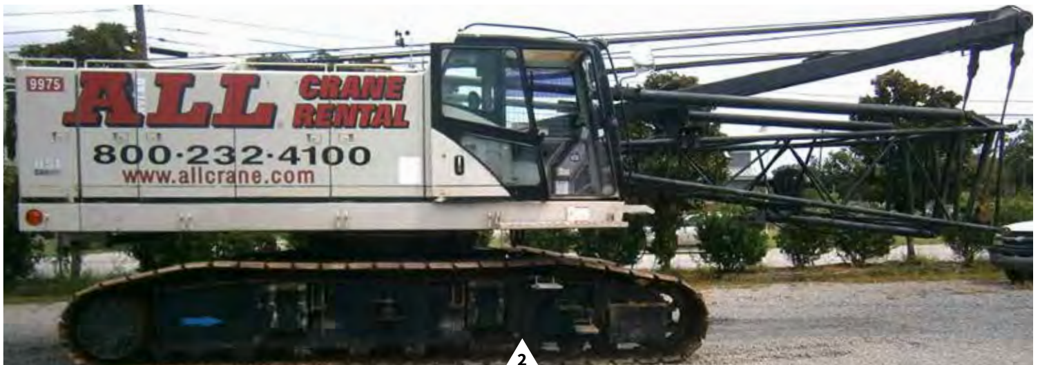
Link-Belt LS218HSL S/N N6J8-0084 , 2008, 110 USt, Isuzu Diesel, 150' Main Boom, 2 Drums, Free Fall. Located in Atlanta, GA. Unit #9975. $495,000.00
