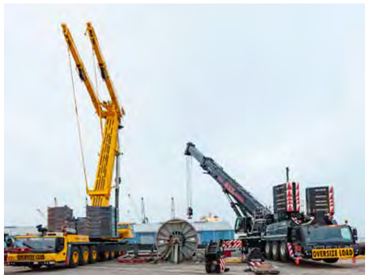
The MegaWingLift™ attachment increases capacity of the GMK7550 for a boost of power.
