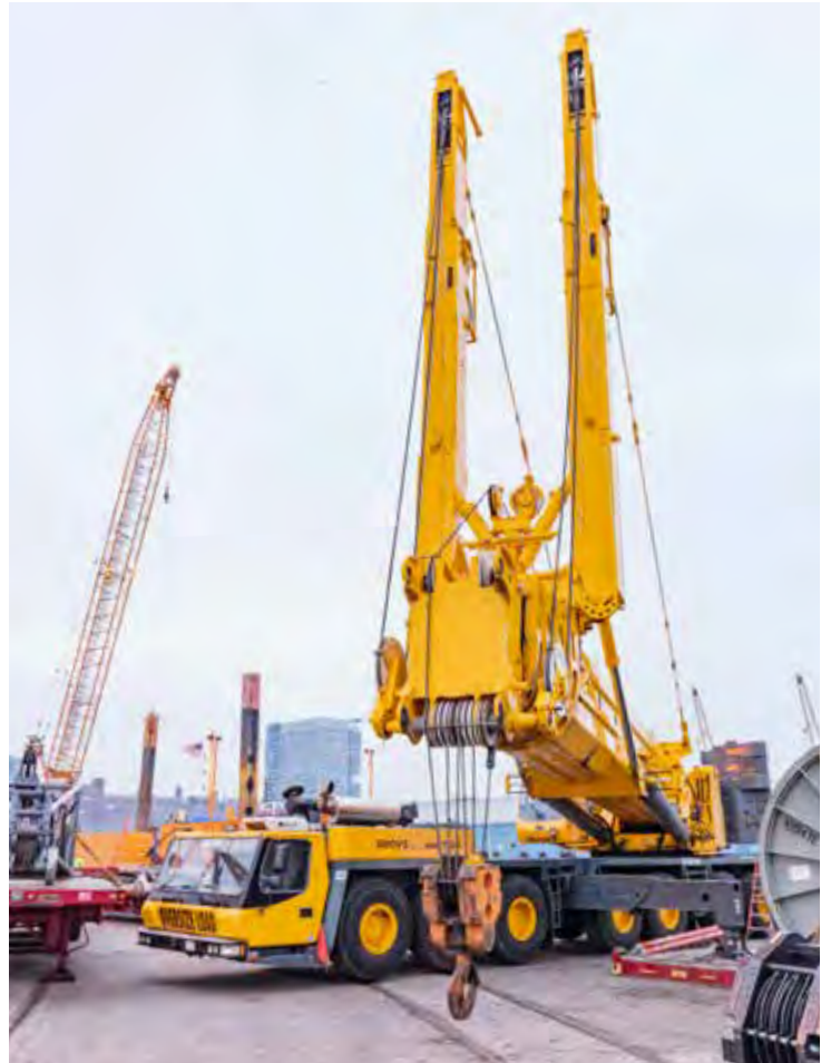
The MegaWingLift™ attachment increases capacity of the GMK7550 for a boost of power.
