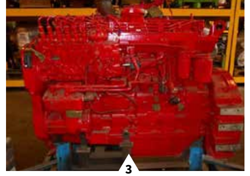
Cummins 6C-8.3 , S/N 46856236, 250 HP @2200, tier 1 NEW/used stage II, 1950lbs. POR
