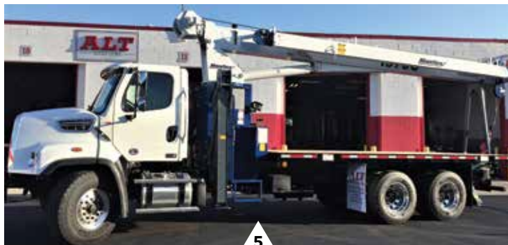
NEW Manitex 1970C , 19 USt, 70' Main Boom, 24' - 41' Jib, Front Bumper Stabilizer for 360° Load Chart Mounted on a Freightliner 108SD. Unit #R1923. Located in Richfield, OH.
