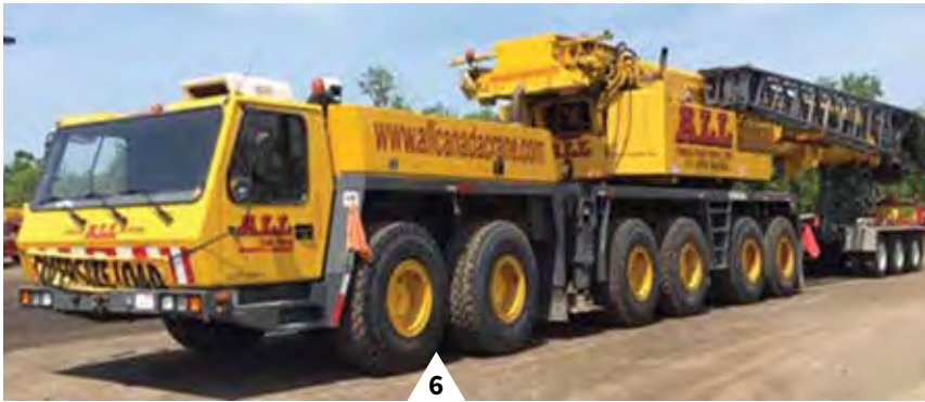
Grove GMK6250L, S/N 6220-9059 (2003), 250 USt, Cummins Diesels, 236' Main Boom, 43'-124' Jib, Aux Hoist, 20.5R25 Tires, A/C, Boom Float Kit, Boom Removal Kit, Hydraulic Quick Disconnect for Outrigger Beams, Boom Dolly, Block and Ball. Located in Elk Mound, WI. $729,000
