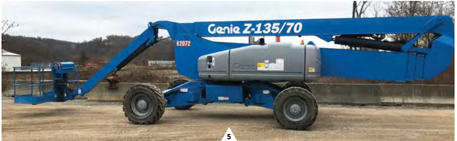
Genie Z-135/70, S/N Z13508-638 (2008) Deutz Diesel Engine, Foam-Filled Tires, 135' Articulating Boom, 4x4. Unit# K2072. Located in Pittsburgh, PA. $67,500
