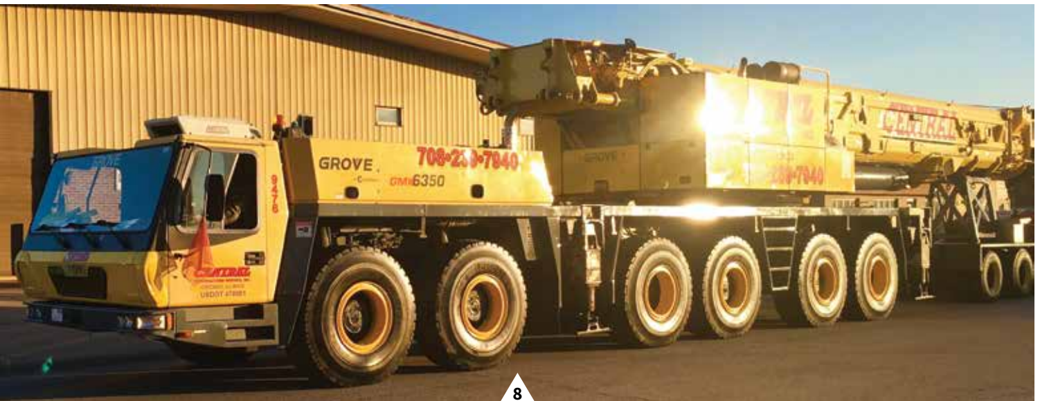
Grove GMK6350, S/N 6300-9099 (2006), 350 USt, Mercedes Diesels, 197' Main Boom, 200' Luffing Jib, 11.5FT offset angle adapter, Aux Hoist, 20.5R25 Tires, A/C, Boom Removal Kit, Hydraulic Disconnect for Outrigger Beams, Removable Rear Outrigger Box, Boom Dolly Block and Ball. Unit #9476. Located in Chicago, IL. $950,000
