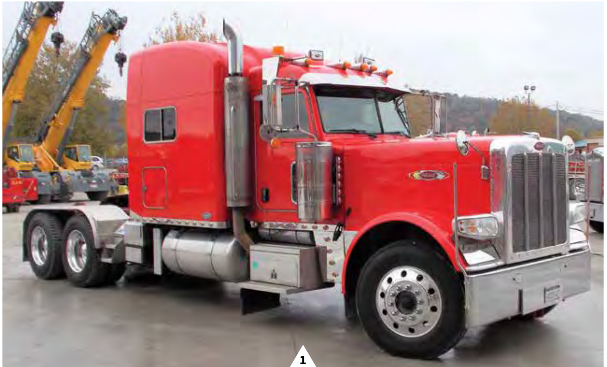
Peterbilt 389 SX (2009) 600 HP, Fuller RTL018918B 18 Speed, Cruise Control on Shift Lever, Double Frame, Holl Air Slide Fifth wheel, 14,600 lb front Axle, 46,000 Rear, Air Trac 46,000 lbs, Painted Aluminum Air Tanks, Aluminum Wheels, Dual 120 Gal Fuel Tank BOC, Platinum Interior, Moto-Mirrors, and much more. POR
