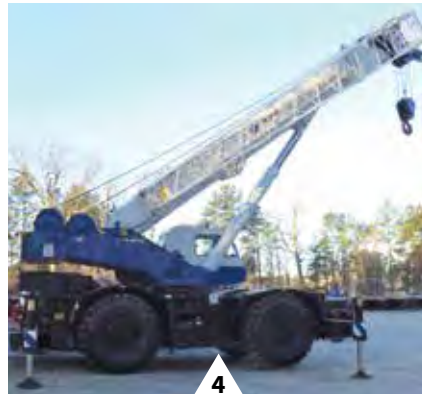
Tadano TR600XXL, S/N 545659 (2004) 60 USt, Mitsubishi 6M60-TLA3B Diesel, Auto Trans, 144' Main Boom, 33'-58' Bifold Jib, Aux Hoist. Unit #8863. Located in Raleigh, NC. $165,000
