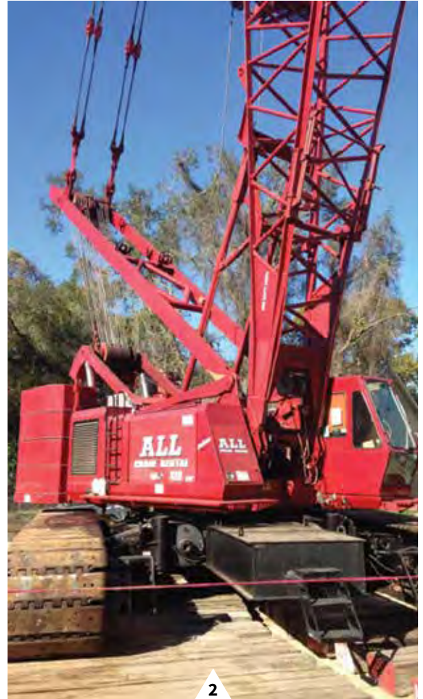
Manitowoc 888: S/N 8881241 (1999), 230 USt, Cummins M11 Turbo Diesel, 200' Main Boom, 40' Jib. Unit #9178. Located in Orlando, FL. Call
