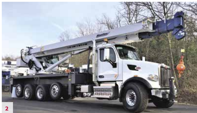
NEW Manitex 40124SHL , 40 USt, 124' Main Boom, 2 piece Jib 30.5'-55', Radio A2B, Heat and A/C in Operator's Cab, Front Bumper Hyd Stabilizer for 360° Load Chart, 10' Steel Bed. Mtd on a Freightliner 114SD 5 Axle Chassis, Cummins X12/475 HP, Allison Trans, Federal Bridge Legal, Air Disc Brakes, 80 Gallon Fuel Tank, and MUCH MORE. (Stock Photo) Unit #R2370
