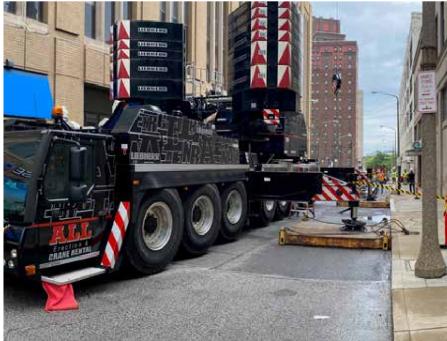
The Liebherr LTM 1450 with versatile VarioBase® outriggers move in close for tight city work, avoiding sidewalk-setup and the consideration of utilities beneath.
