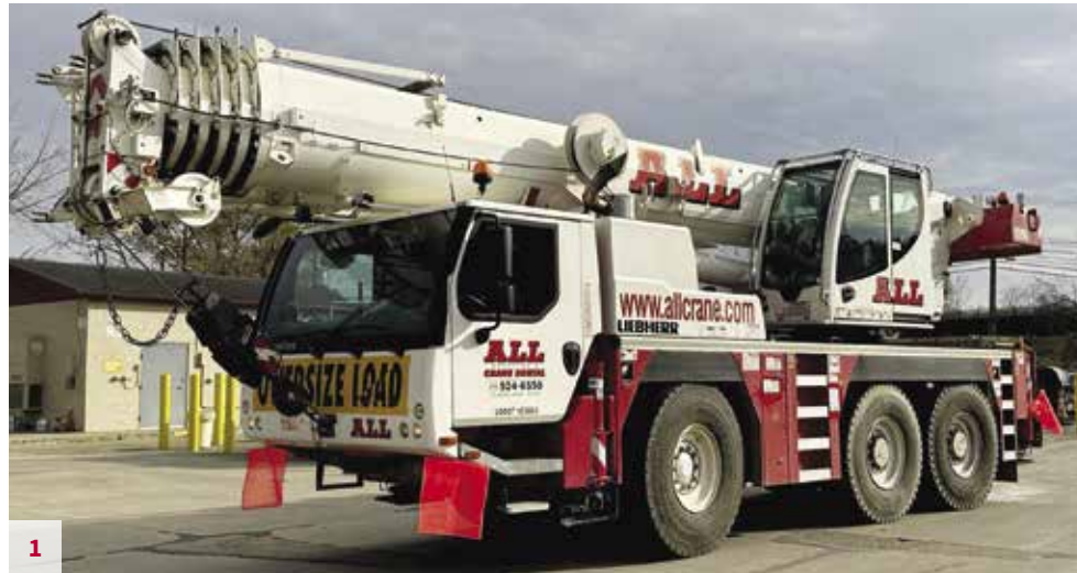
1 Liebherr LTM 1060 3.1 - S/N 058142, 2016 , 50 USt, 6 x 4 Drive, Liebherr Diesel, 6,842 Hours and, 54,491 KM, 157' Main Boom, 31'-52' Swing Away Jib, Rooster Sheave, Aux. Hoist, Engine Independent Heater, 445/95 R25 Tires, Vario Base, Battery Charger, 28,160 lbs of Counterweight, Working Floodlights, Flight Warning Light, Wind Speed Indicator, Block and Ball. Located in Cleveland, OH. Unit #11194 $707,000
