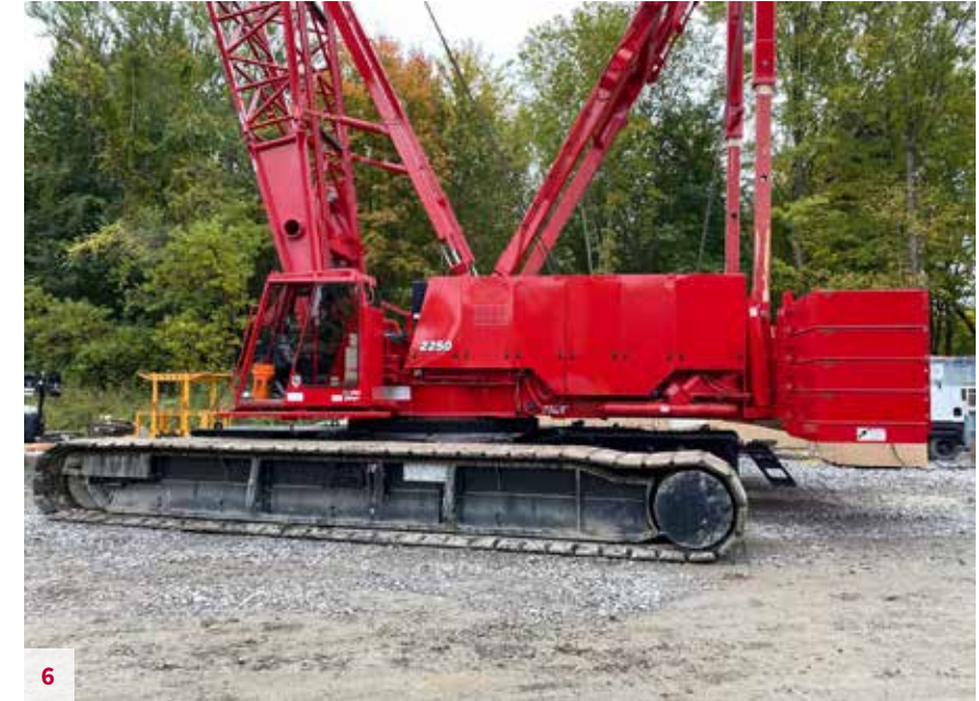
Manitowoc 2250 - S/N 2251390 , 2014, 300 USt, Cummins QSX15 Tier4i (11,512 Hours), 200' Main Boom, Self Erect, Auto-lube for Turntable and Crawlers, Wind Anemometer, Series 2 and 3 Counterweights, A/C, Maxer 2000 Prepped, Liftcrane Lagging Grooved 1-1/8 on Left and Right Drum, Detachable Upper Boom Point, Cold Weather Package, Block and Ball. Located in Cleveland, OH. Unit #10923 $1,665,000
