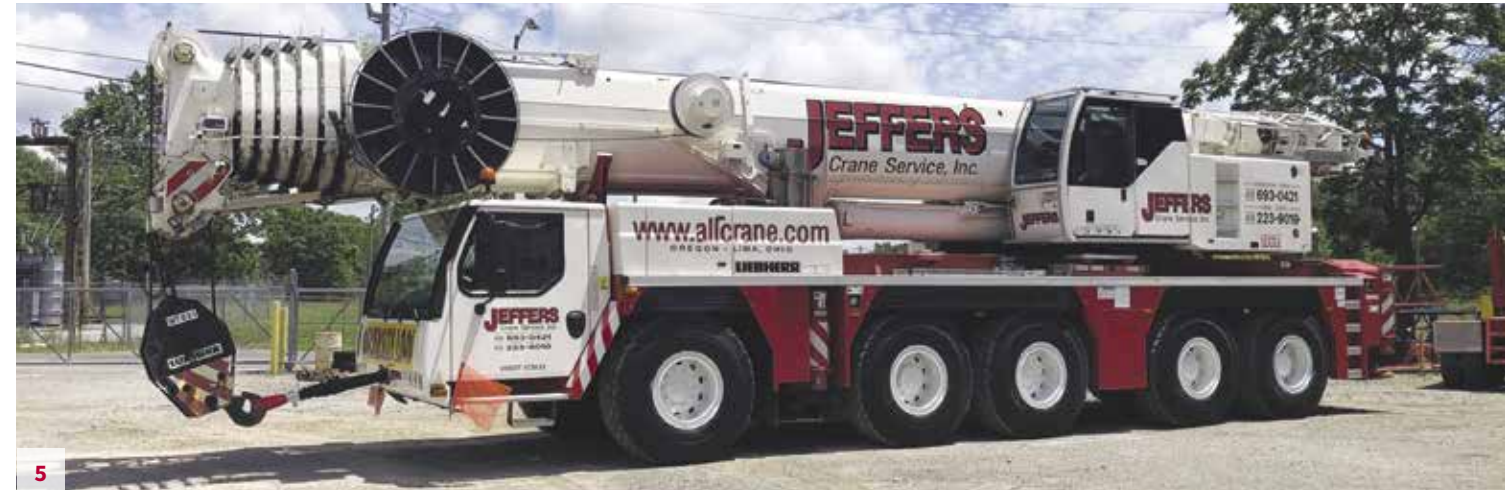
5 Liebherr LTM 1200 5.1 - S/N 093397, 2013 , 240 USt, Liebherr Diesels, 10,862 Upper Hours, 4,621 Lower Hours, 49,868 KM, 236' Main Boom, 40'-72' Hydraulic Swingaway Jib, (2) Jib Inserts, Aux. Hoist, 20.5 R25 Tires, A/C in Upper and Lower Cabs, Working Floodlights, Liccon, Block and Ball. 3 Axle Boom Dolly. Located in Lima, OH. Unit #10691 $1,239,000
