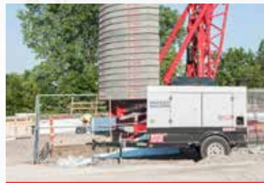
Adaptable to multiple power sources: site power, generator, or AC power. (230-volt single phase or 480-volt three phase.)
