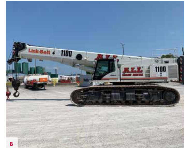
Link-Belt TCC1100 - S/N S1K4-4109 , 2014, 110 USt, Cummins Diesel (8,339 Hours), 150' Main Boom, 10'-31'-55' Jib, Aux. Hoist, Upper Mount Work Lighting, Single Axis Controls, Toolbox, Rotating Beacon Light, Aux. Lifting Sheave, RCL Light Bar, Block and Ball. Located in Baton Rouge, LA. Unit #10868 $775,000
