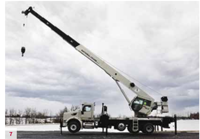
NEW National NBT45127-2 , 45 USt, 127' Main Boom, 31'-55' Jib, Internal A2B ATB, Updated Operator Cab, Max counterweight package, Single Front Outrigger, and much more. Mtd on a Peterbilt 567 Chassis, X-15/500 HP, 18-Speed UltraShift Plus Trans, Federal Bridge Legal, 100 Gallon Fuel Tank with Heater, and MUCH MORE. Multiple Units Available throughout 2023. EXW Richfield, OH. (Stock Photo) Unit #R2380
