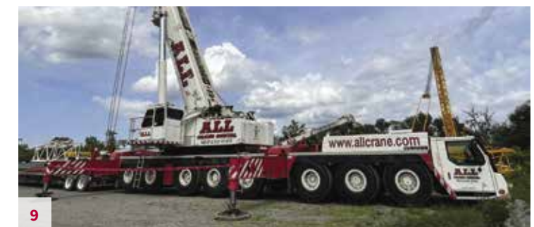
9 Liebherr LTM 1500 8.1 - S/N 095255, 2012 , 600 USt, Liebherr Tier 3, 7,502 Upper Hours, 2,635 Lower Hours, 40,702 KM, 276' Main Boom, 298' Luffing Jib, Y-Guy, 2 Winches, 20.5 R 25 Tires, A/C, 8 Counterweight slabs each with 16,500, Removable Telescopic Boom, Additional Fuel Tank, Telma Brake, Working Lights, Liccon, Special Design and Assembly for Nelson Boom Launching Lugs, Blocks and Ball. Located in Fort Wayne, IN. Unit #10518 $2,995,000
