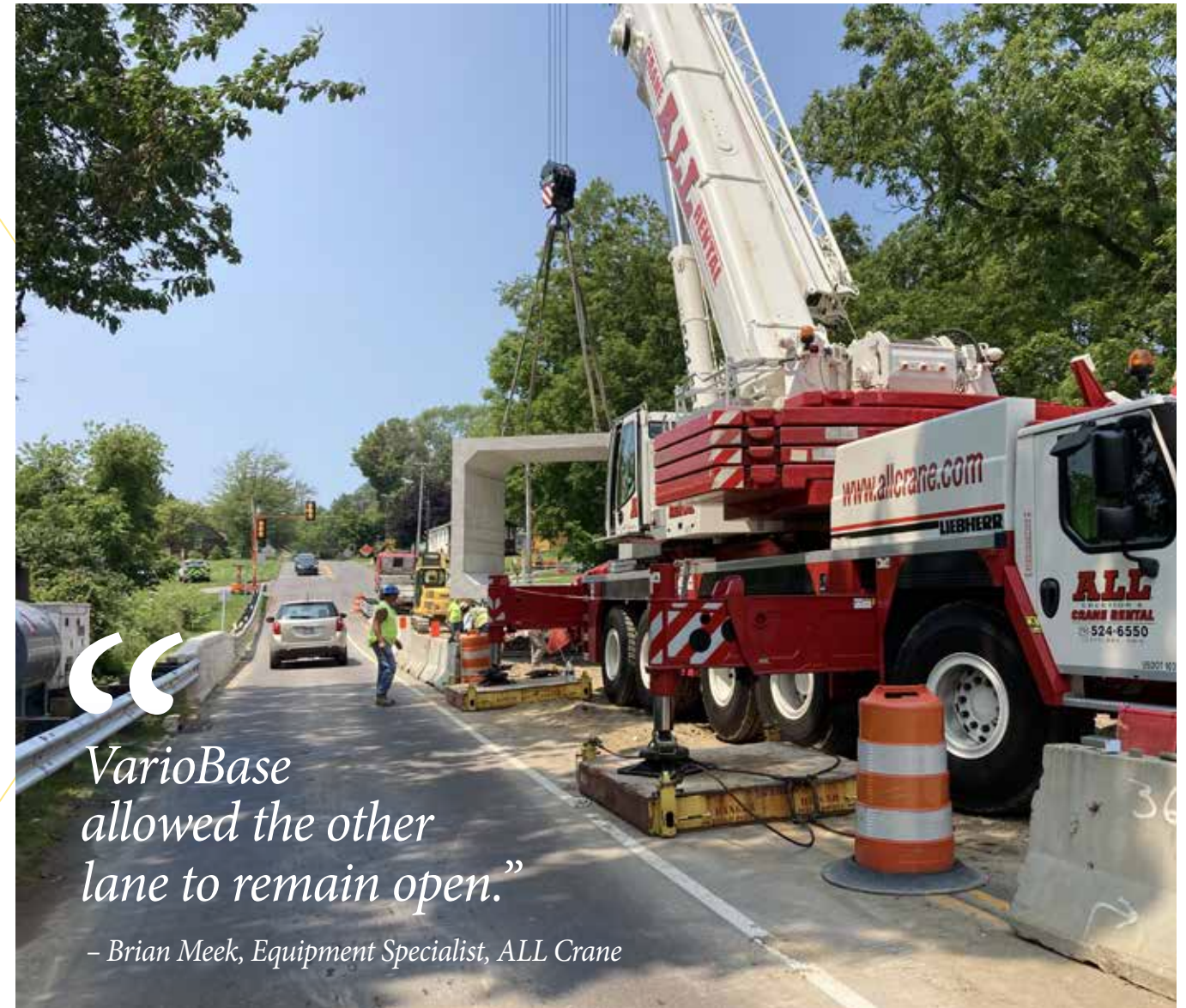
VarioBase allowed ALL's Liebherr LTM 1160-5.2 crane to get the job done while keeping a lane of traffic open.
