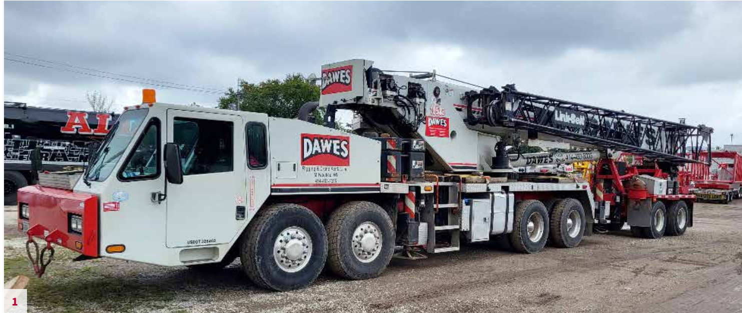
Link-Belt HTC-8690 - S/N N3K3-3148 , 2013, 90 USt, Cummins ISX11.9, 13,786 Hours, 70,674 Miles, 140' Main Boom, 35'-58' Offset Jib, Aux. Hoist, Daytime Running Lights, Amber Strobe, Trailer Air & Electric, 39,500# Counterweight, 2 Speed Winches, Winch Rollers, RCL Light Bar, Upper and Lower A/C, Single Axis Controls, Upper Storage Box, Aux. Lifting Sheave, Boom Flood Lights, Boom Float Kit, Block and Headache Ball. Located in Milwaukee, WI. Unit #10583 $529,000
