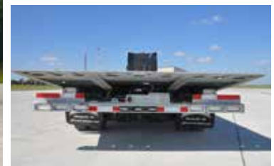
Landoll 455B-53 , Trailer Standard Equipment, Deck Rating: 70,000 Lbs. in 10', Capacity: 110,000 lbs., Main Frame: Fabricated 80,000 & 100,000 PSI Yield, 40" Center, Four Beam Design, Cross members: Alternating 4" I-Beam on 8" Centers, Tires: 235/75R 17.5 LRH Double Coin, Rims: 17.5x6.5 Tubeless, Axles: 3-25,000 lb. Dual Tire Oil Bath Bearings, Suspension: Neway Air Ride 22,500 Lb. Capacity, Brakes: 12.25x7.5 Full Air/Brakes ABS 4s/2m POR
