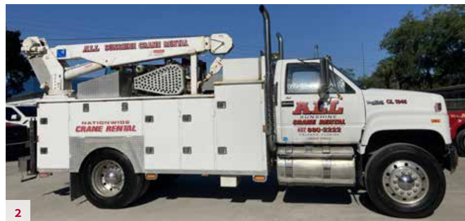
GMC Topkick , 1994, Southern Truck, Diesel Cat 3116, 35,000 GVW, Auto Crane 8005H, Miller Bob Cat 225 Welder, Manual Transmission. POR
