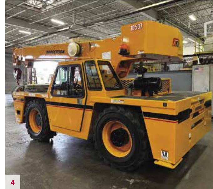
4 Broderon IC-200-3G - S/N 219063200, 2012, 15 USt, Cummins B3.3 (6,962 Hours), 50 Main Boom, 16 Jib, 2 Wheel Drive and 4 Wheel Steer, Engine Heater, Headlight and Taillight Grilles, Strobe Light, All Weather Cab, RCL Greer, Block and Ball. New Paint. Located in Cleveland, OH. Unit #10507 $119,000
