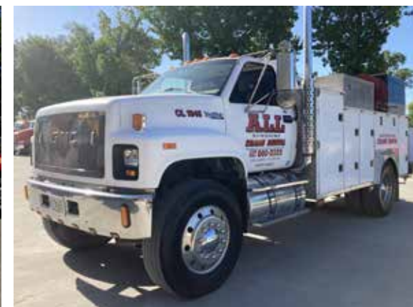
GMC Topkick , 1994, Southern Truck, Diesel Cat 3116, 35,000 GVW, Auto Crane 8005H, Miller Bob Cat 225 Welder, Manual Transmission. POR
