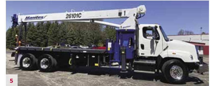
NEW 2023 Manitex 26101C , 26 USt, 101' Main Boom, 29' Jib, Rotation Resistant Rope, Continuous Rotation, Front Bumper Hyd Stabilizer for 360° Load Chart, Out & Down Outriggers, Oil Cooler, Bulkhead, and Extra Control Valve for an accessory. Mtd on a Freightliner 114SD+ Chassis, Cummins X12/455 HP, Allison 4500 Trans, 20K FA, 40K Tandem, Air Disc Brakes, 100 Gallon Fuel Tank, and Backup Camera. (Stock Photo) Unit #R2412
