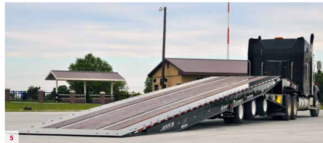
Landoll 455B-53 , Trailer Standard Equipment, Deck Rating: 70,000 Lbs. in 10', Capacity: 110,000 lbs., Main Frame: Fabricated 80,000 & 100,000 PSI Yield, 40" Center, Four Beam Design, Cross members: Alternating 4" I-Beam on 8" Centers, Tires: 235/75R 17.5 LRH Double Coin, Rims: 17.5x6.5 Tubeless, Axles: 3-25,000 lb. Dual Tire Oil Bath Bearings, Suspension: Neway Air Ride 22,500 Lb. Capacity, Brakes: 12.25x7.5 Full Air/Brakes ABS 4s/2m POR
