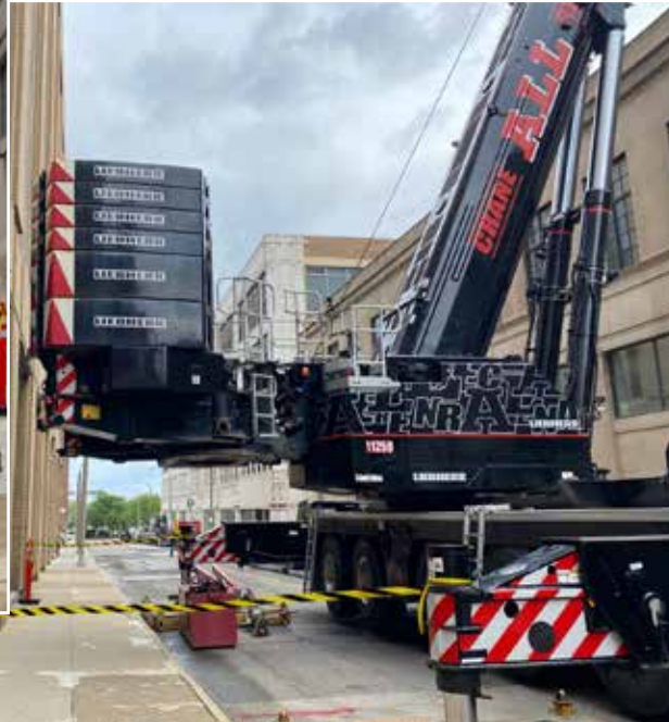
The Liebherr LTM 1450 with versatile VarioBase® outriggers move in close for tight city work, avoiding sidewalk-setup and the consideration of utilities beneath.
