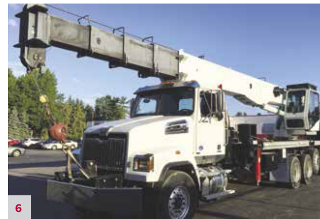
Elliott 36127R , 36 USt, 127' Main Boom, Jib Ready, Aluminum Deck, Single Sheave Block, and Ball. Mtd on a Western Star W4700 Chassis, DD13 470 HP, Allison Transmission, Dual 50 Gallon Fuel Tanks. Unit #U2225
