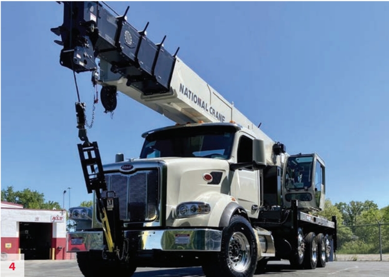
NEW National NBT45127-2 , 45 USt, 127' Main Boom, 31'-55' Jib, Front Bumper Stabilizer for 360° Load Chart, Internal A2B, and Max cwt. Mtd on a Peterbilt 567 chassis, X15/500 HP, 18-Speed Ultrashift Trans, Federal Bridge Legal, 100 Gallon Fuel Tank, Locking Rear Axles, and Wheel Ends, Alum Wheels, AM/FM Radio, Bluetooth Capable, and MUCH MORE. (Stock Photos) Unit #R2378
