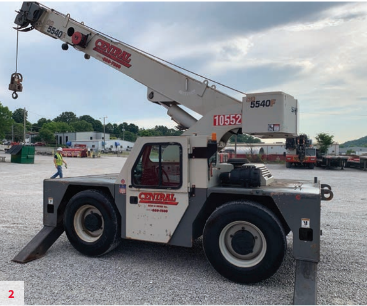
Shuttlelift 5540F - S/N 321881 , 2012, 15 Ton, Cummins QSB3.3, 3,926 Hours, 41' Main Boom, 15' Offsettable Jib, 2 Wheel Drive, 4 Wheel Steer, Enclosed Cab, Lifting and Tie Down Lugs, Load Indicator, Strobe Light, Headlight and Taillight Grilles, Cab Dome Light. Located in Phoenix City, AL. Unit #10552 $85,000
