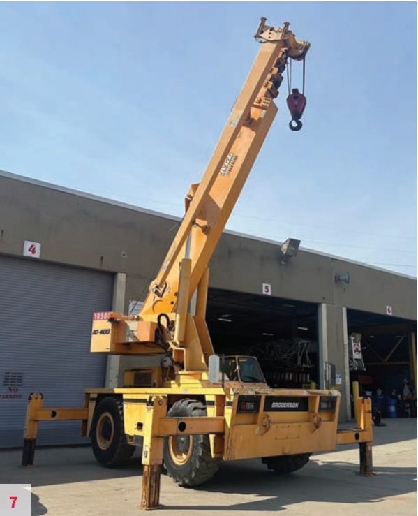
Broderick IC-400-3A, S/N 14031400 , 2014 25 Ton, Cummins QSB 4.5 Tier 4i, 4,015 Hours, Catalytic Converter, 64' Main Boom, 20' Offset Jib, 17.5 x25, 20ply Tires, Control System with Joysticks, Rear-view Mirror, All Weather Cab, Air Conditioning, Windshield Washer, Strobe Light, Rated Capacity Limiter, Hoist Drum Rotation Indicator, Block and Ball. Located in Toledo, OH Unit #10986 $227,000
