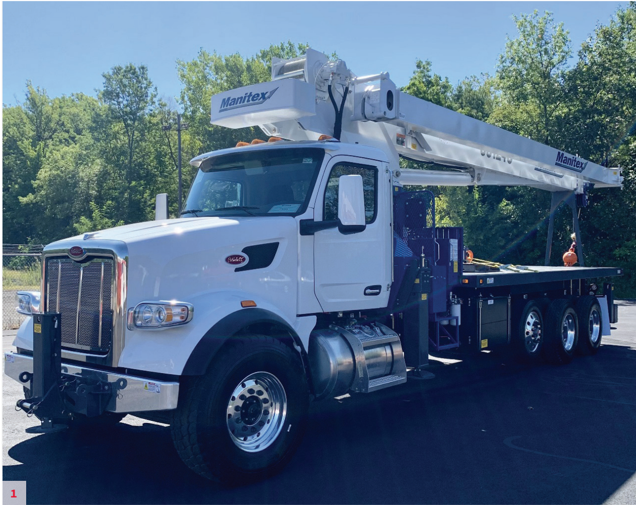
NEW Manitex 35124C , 35 USt, 124' Main Boom, 31' Jib, Front Bumper Stabilizer for 360° Load Chart, Out & Down Outriggers, Oil Cooler, and Continuous Rotation. Mtd on a Freightliner 114SD+, Cummins X12 500HP, Allison 4500 Trans, 100 Gallon Fuel Tank, Air Disc Brakes, Federal Bridge Legal, and MUCH MORE. (Stock Photo) Unit #R2489
