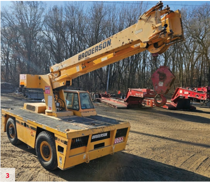
Broderick IC-80-3J - S/N 65796680 , 2013, 9 USt, Cummins B3.3 L Diesel (4,148 Hours), 30' Main Boom, 10' Jib, Catalytic Converter, Engine Heater, 4 Wheel Steer and 2 Wheel Drive, Pneumatic 10.00 x 15 Tires, All Weather Cab, A/C, Strobe Light, Hoist Drum Rotation Indicators, RCL Greer, Block and Ball. Located in Kaukauna, WI. Unit #10683 $78,500
