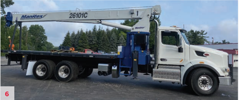
NEW 2023 Manitex 26101C , 26 USt, 101' Main Boom, 29' Jib, Rotation Resistant Rope, Continuous Rotation, Front Bumper Hyd Stabilizer for 360° Load Chart, Out & Down Outriggers, Oil Cooler, Bulkhead, and Extra Control Valve for an accessory. Mtd on a Freightliner 114SD+ Chassis, Cummins X12/455 HP, Allison 4500 Trans, 20K FA, 40K Tandem, Air Disc Brakes, 100 Gallon Fuel Tank, and Backup Camera. (Stock Photo) Unit #R2412
