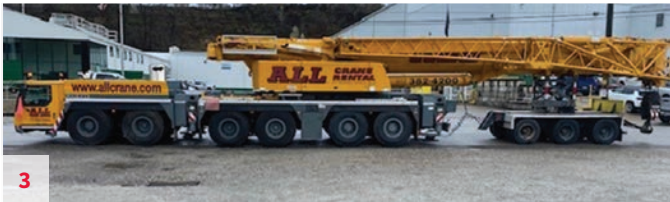
Liebherr LTM1250 6.1 - S/N 070980 , 2013, 300 Ton, Liebherr Diesels, 8,512 Upper Hours, 4,970 Lower Hours, 74,234 Miles, ZF Trans, 236' Main Boom, 40' - 70' Swingaway Jib, (2) 23' Jib Inserts, Aux Hoist, 214,500 lbs of Counterweight, Removable Main Boom, Removable Rear Outrigger Boxes, Air Conditioning, Blocks and Ball. 3 Axle Boom Dolly. Located in Pittsburgh, PA. Unit #10668 $1,509,000
