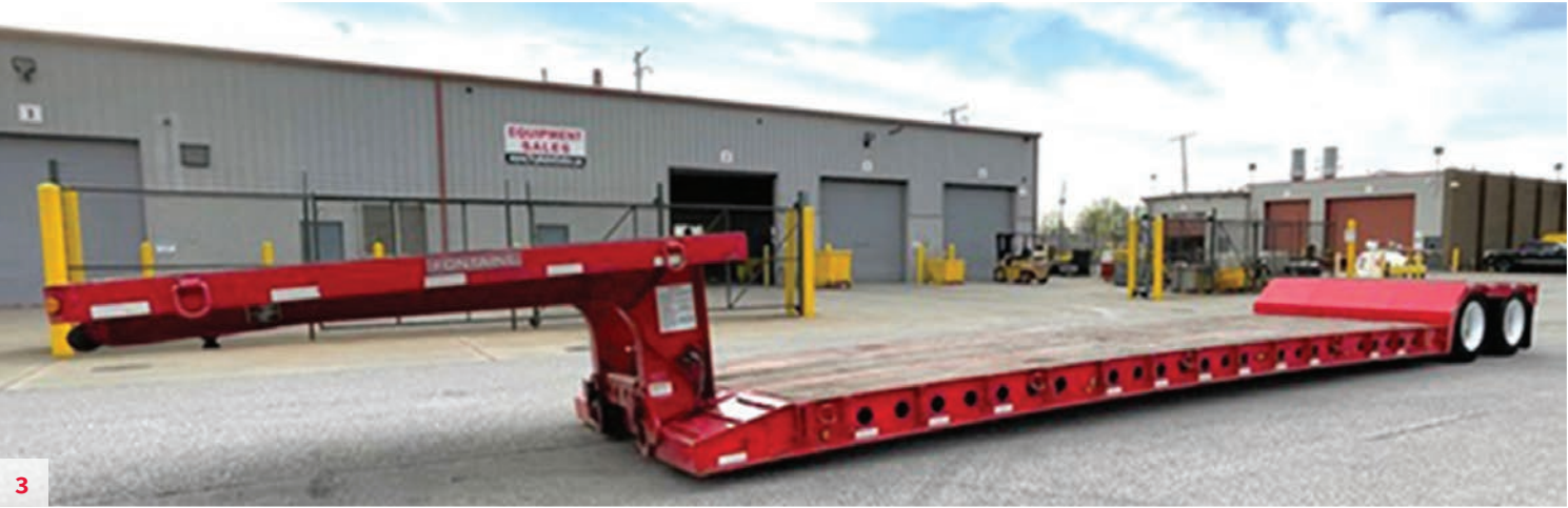
Fontaine RGN Mechanical , 2007, Air Ride, Mechanical Detach, 4th Axle Pin on Option, Ready to work, Some minor rust scale below, Sold as is, Inspections welcome. Unit #X097 POR
