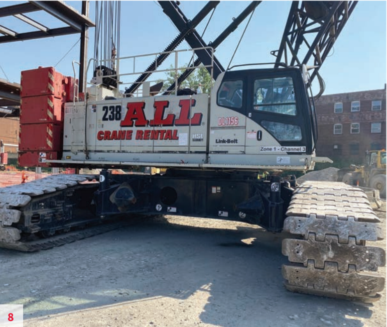
Link-Belt LS238HSL - S/N P5K2-2842 , 2012, 150 Ton, Isuzu 6HKI T4I, 20,376 Hours, 180' Main Boom, 40' Jib, 3rd Drum, Free Fall, Full Counterweight, Block and Ball. Located in Cleveland, OH. Unit #DL1156mlw $700,000
