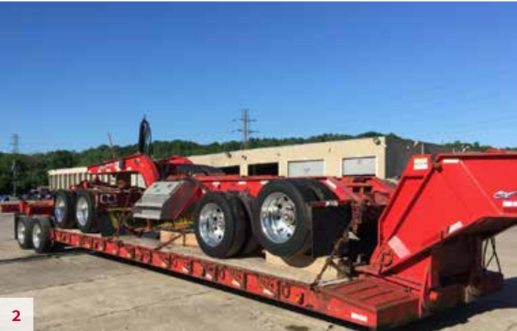
Talbert 60 TON 2+2+2 Multi Axle Trailer 1989, Turner Air Suspension, 73' 5" Overall Length, 9' 3/4" Width, 27'-5" Well, Talbert Telescopic Drop Legs, Tool Boxes, Weigh Load Scales, Aluminum Wheels, 45" Wide Beam, 50,000-lb Empty Weight, Well-Maintained. EXW Cleveland, OH. Unit #X392. POR
