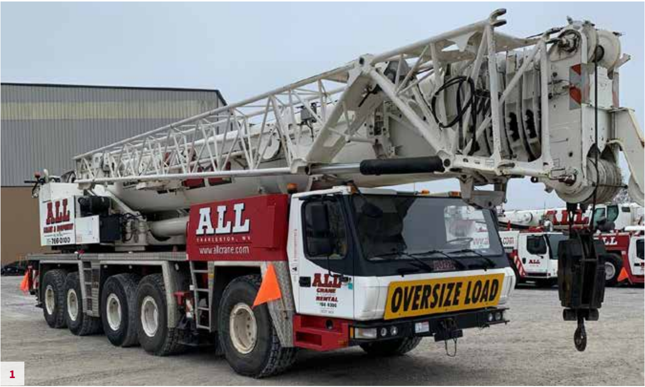
Grove GMK5225, SS/N 5170-3003 2009, 225 USt, Cummins Diesels, (9,125 Upper Hours/4,975 Lower Hours), 117,000 KM, Allison Transmission, 210' Main Boom, 36'-59' Bifold Swingaway Jib Hydraulic Offset, (2) 26' Jib Inserts, Aux Hoist, 10x8 Drive In Leiu of Std 10x6, 20.5 R25 Tires, Boom Float Kit, Boom Removal Kit, A/C in Upper and Lower, Hydraulic Disconnect for All Outrigger Beams, 2 Axle Boom Dolly. Located in Charleston, SC. Unit #10281. $647,000
