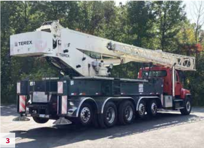
2016 Terex Crossover 4500L 45 USt, 129' KEEL Main Boom, 32' -49' Offset Able Jib, X Pattern Outriggers, Anemometer, Removable Front Window in Operators Cab, Worklight Package, Dual Axis Controls, Rotation Resistant Cable, Winch Camera, Heat & A/C, Mtd on a Freightliner 114SD Chassis DD13 450 HP, 8LL Trans, 20K F/A 46K R/A, Three 10,000 lb lift Axles (One Tag and Two Pushers), Federal Bridge Law Legal. EXW Richfield, OH. Unit #U2116. POR
