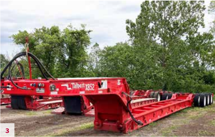
Talbert 45 TON 3 Axle Trailer 2000, Air Ride Suspension, 255/70R22.5 Wheels, 54'-8" Overall Length, 27'-1" Open Well, 45" Wide Beam, 60" Axle Spacing, Hydraulic Tank Located on Trailer, Refurbished and Ready to Work. EXW Cleveland, OH. Unit #X852. $53,485
