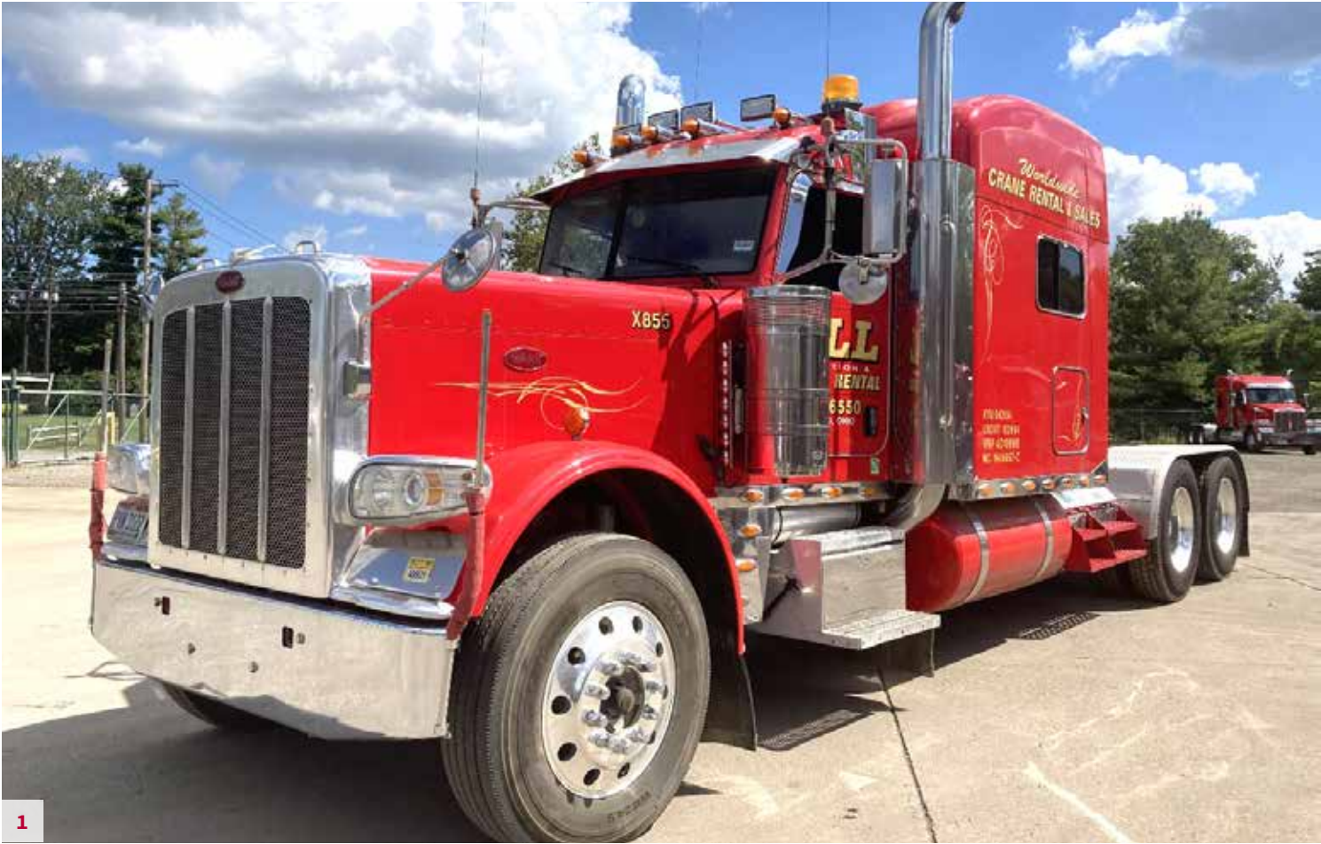
Peterbilt 389 3 Axle Sleeper 2010, 14,320-lb Front Axle, 46,000-lb Rear Axle, Cummins ISX15 600HP HP, Fuller 18-speed Transmission, Peterbilt Air Trac, 46,000 lbs Steel Susp Insert, 10-3/4" Steel Rails to 354" Holland Fifth Wheel, Top Plate Diff Lock, Heavy Wall Drive Axles, Premium Air Cleaners, Dual Exhaust, Painted Aluminum Air Tanks, Aluminum Wheels, Dual 135 Gal Fuel Tanks, Fuel Heaters, Full Gauges, Thermal Insulation Pkg., Woodgrain Panels, Strobe Lite. EXW Cleveland, OH. Unit #X855 POR
