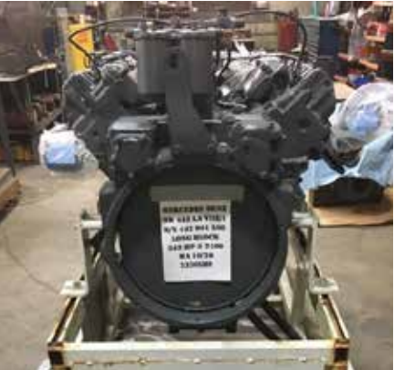
Mercedes Benz OM442 LA VIII/1 Engine Part #UNQMBOM442, S/N 442 901 506, Long block, 543 HP @ 2100, 2,330 lbs, MA 10/20. POR
