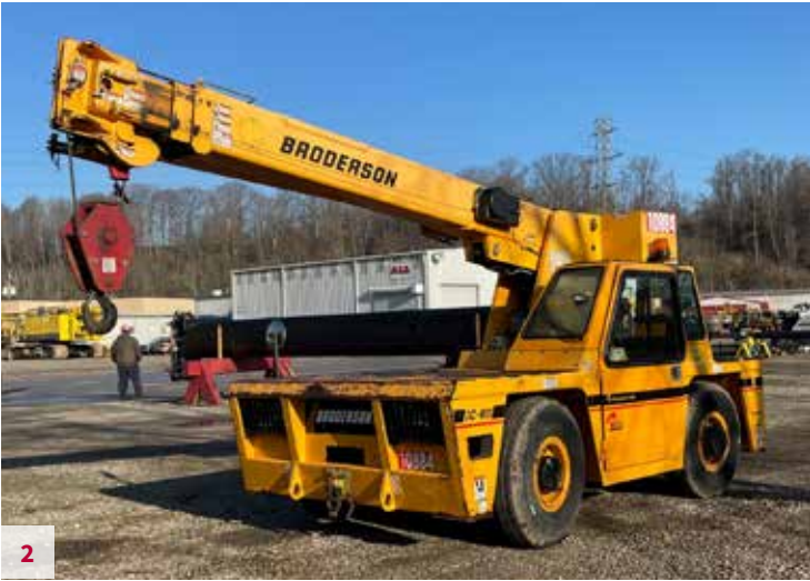
Broderson IC-80-3J, S/N 67132380 2013, 9 USt, Cummins B3.3 L Diesel (5,800 Hours), Catalytic Convertor, Engine Heater, 4 Wheel Steer and 2 Wheel Drive, 30' Main Boom, 10' Jib, Pneumatic 10.00 x 15 Tires, All Weather Cab, A/C, Strobe Light, Hoist Drum Rotation Indicators, RCL – Greer. Located in Pittsburgh, PA. Unit #11263. $83,500
