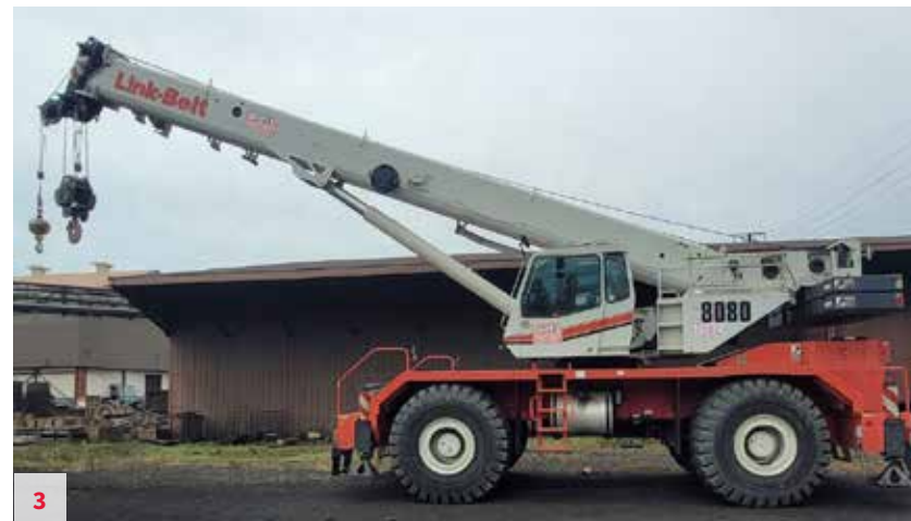
Link-Belt RTC-8080 - S/N S4K3-3435 , 2013, 80 USt, Cummins QSB6.7 (8,507 Hours), 127' Main Boom, 10'-38'-64' Offset Jib, Aux. Hoist, 19,200# Counterweight, RCL Bar Graph, A/C, Joystick Controls, Block and Ball. Located in Hammond, IN. Unit #10774 $307,000
