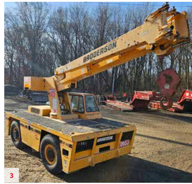
3 Broderon IC-80-3J - S/N 65796680 , 2013, 9 USt, Cummins B3.3 L Diesel (4,148 Hours), 30' Main Boom, 10' Jib, Catalytic Converter, Engine Heater, 4 Wheel Steer and 2 Wheel Drive, Pneumatic 10.00 x 15 Tires, All Weather Cab, A/C, Strobe Light, Hoist Drum Rotation Indicators, RCL Greer, Block and Ball. Located in Kaukauna, WI. Unit #10683 $83,500
