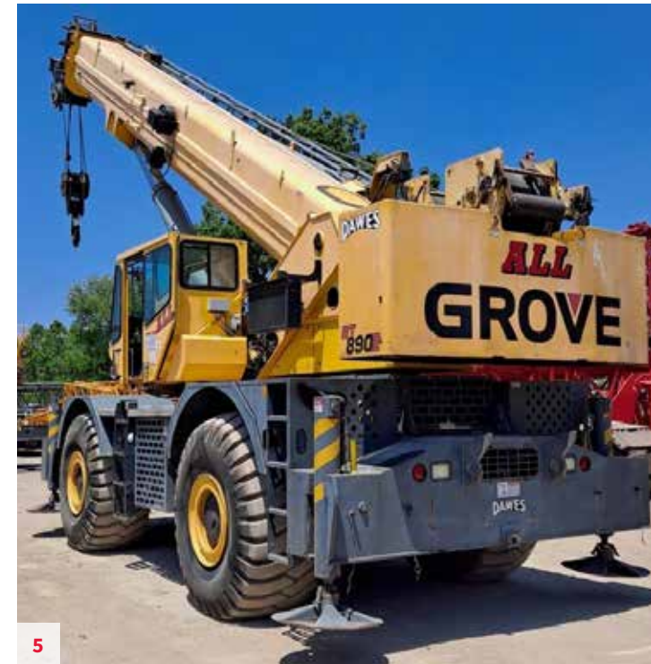
Grove RT890E - S/N 229891 , 2009, 90 USt, Cummins QSB 6.7L (13,864 Hours), 142' Main Boom, 33'-56' Jib, Aux. Hoist, A/C, Valve Package, Block Heater, Block and Ball. Located in Kaukauna, WI. Unit #10224 $199,000
