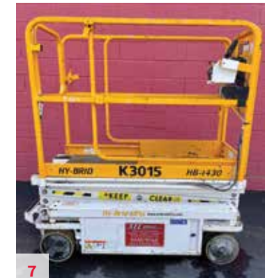
7 Hy-Brid HB-1430, S/N D02-11829 , 2016, 14' Platform Height, DC, Non-Marking Tires, 2x4. Located in Richfield, OH. Unit #K3015 $4,000
