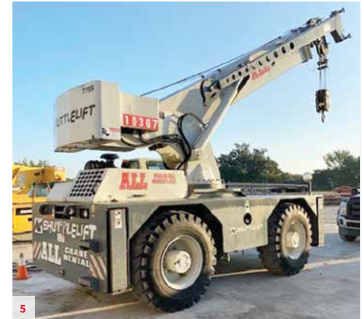
5 Shuttlelift 7755 - S/N 321441 , 2010, 22 USt, Cummins QSB 4.5 (10,736 Hours), 67' 5" Section Boom, 17' Jib, 4 Wheel Drive, 17.5-25 Bias Tires, LMI, Enclosed Cab, Cold Start Kit, Engine Block Heater, Full Lighting Package, Outrigger Alarm System, Headlight and Taillight Grilles, Lifting and Tie Down Lugs, Block and Ball. Rebuilt Scope Cylinder 2023. Located in Cleveland, OH. Unit #10367 $173,000
