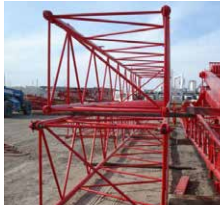
777 Luffing Jib PN 777Luffingjib, Complete Luffing Jib to fit Manitowoc 777 crawler crane. No 139 Jib-170'. POR
