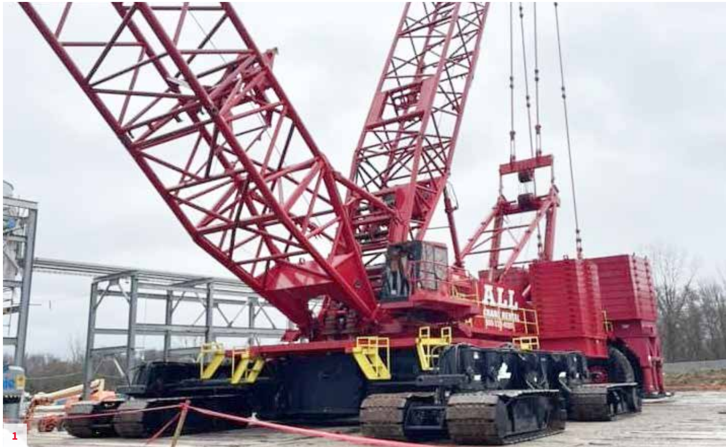
Manitowoc 21000 - S/N 21001007 , 2001, 1000 USt, Cummins QSK19-C600, 300' #80 Main Boom, 280' #81 Luffing Jib (S/N 21005006), 140' Mast, MAX-ER Attachment (S/N 21003006), New Rotec Bearing (2019), Block and Ball. Located in Columbus, OH. Unit #9466 $1,900,000
