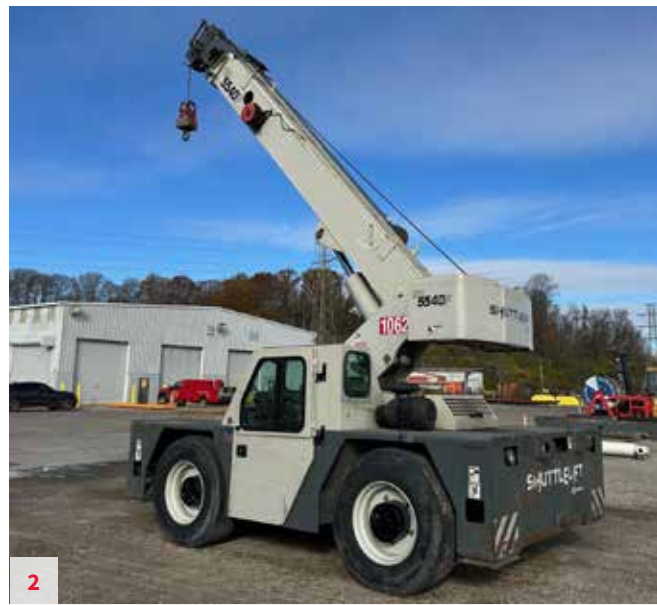
2 Shuttlelift 5540F - S/N 322010 , 2012, 15 USt, Cummins QSB3.3 (2,578 Hours), 41' Main Boom, 15' Jib, 2 Wheel Drive, 4 Wheel Steer, Enclosed Cab, Lifting and Tie Down Lugs, Load Indicator, Heater, Strobe Light, Headlight and Taillight Grilles, Cab Dome Light, Block and Ball. Located in Cleveland, OH. Unit #10624 $87,500
