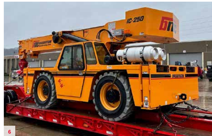
6 Broderon IC-250-3E - S/N 77438250 , 2023, 18 USt, GM5.7L V8 EPA Tier II LPG Fuel Only, (374 Hours), 50'1" Main Boom, 20' Offset Jib, Four Wheel Steer and 4 Wheel Drive, High Traction Tread Non-Marking Tires, Rear Pintle Hook, All Weather Cab (Heater, Defroster, & Wiper), Strobe Light, Boom Work Lights, Rated Capacity Limiter, Drum Rotation Indicator, 4 Part Block and Ball. Located in Indianapolis, IN. Unit #11821 $327,000
