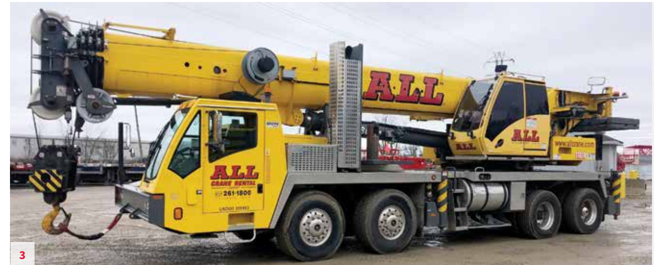
Grove TMS900E - S/N 234862 , 2014, 110 USt, Cummins ISX12 11,359 Hours 78,874 Miles, 142' Main Boom, 33'-56' Bifold Jib, Aux. Hoist, Aux. and Light Package, Trailing Boom Package, XL Counterweight Package, Outrigger Monitoring System, A/C, Block and Ball. Located in Columbus, OH. Unit #11010 $599,000
