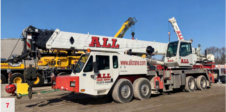
Link-Belt HTC8650 II, S/N L8K3-3589 2013, 50 USt, Cummins EPA 13 Upgrade Diesel, (5,965 Hours), 42,100 Miles, 110' Main Boom, 38.5'-51' Offset Bifold Jib, Aux. Winch, RCL Light Bar, A/C, Block and Ball. Located in Fort Wayne, IN. Unit #10836. $349,000
