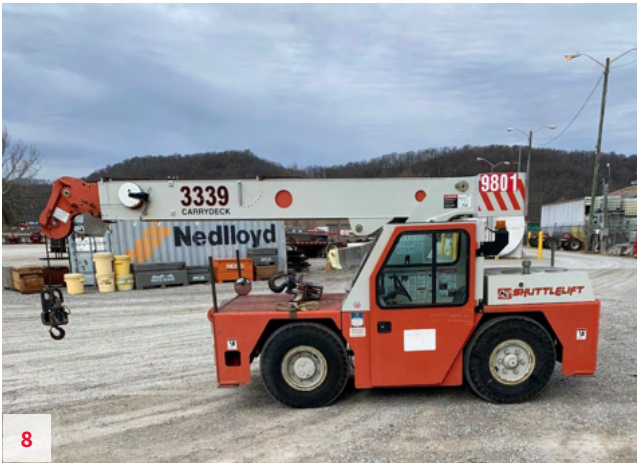
Shuttlelift 3339, S/N 320688 2007, 9 USt, Cummins 4B3.3 Diesel, 1,500 Hours, 32'10" Full Power Boom, 12' Offsettable Swingway Jib, Crab Steer, Heater & Defrost, Lifting and Tie Down Lugs, Headlight and Taillight Grilles, Cab Dome Light, Enclosed Cab, Load Indicator. Located in Knoxville, TN. Unit #9801. $37,500
