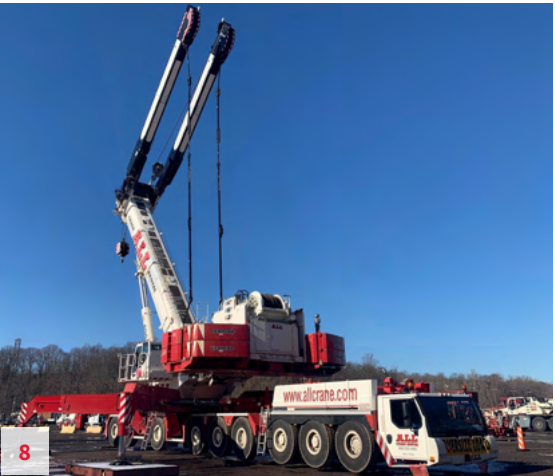
Liebherr LTM 1750-9.1, S/N 096038 2013, 900 USt, Liebherr Diesel Tier 4i, ZF Transmission, (5,358 Upper Hours/2,298 Lower Hours), 22,000 Miles, 171' Main Boom, 20'-180' Fixed Jib, 69'-206' Luffing Jib, V2-32' 8" Lattice Section, V3 - (2) 16' 4" Lattice Section, Eccentric VE includes 16'4" Boom Extension, 2 Winches, 3rd Winch for Luffer, Y Guy, 449,700 lbs of Counterweight, 16.00 R25 Tires, Self-Assembly, Removable Telescopic Boom incl. Luffing Cylinder Disassembly, Quick Disconnect, Removable House, Camera System for Reverse Drive. Located in Indianapolis, IN. Unit #10662. $5,200,000 ExWorks CURRENTLY AVAILABLE
