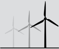
Turbines are getting taller to reach faster, more constant winds higher in the atmosphere. The higher you go, the faster the winds and the more energy can be produced.
