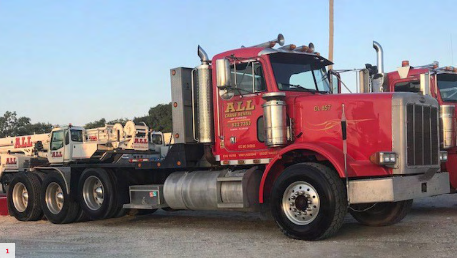
Peterbilt 378 B 4-Axle Day Cab Tractor 1990, 189.5 GAWR Front, 12,860-lb GAWR Rear 46,000-lb Meritor Pusher Axle 17,000-lb, Cummins NTC 444 Hp Eaton Fuller Trans, RTO15618 4.11 Rear Axle Ratio, Steel Susp. Insert, 150-Gal Fuel Tank, RH A/C. EXW Tampa, FL. Unit #CL857.
