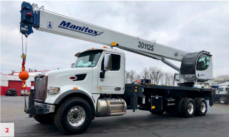
NEW 2022 Manitex 30112S 30 USt, 112' Main Boom, Jib Ready, and Front Bumper Hyd. Stabilizer for 360 Load Chart. Mtd on a Freightliner 114SD Chassis, ISX12/500HP, Allison 4500 Trans, Federal Bridge Legal, Air Disc Brakes, 90 Gallon Fuel Tank, and MUCH MORE. EXW Richfield, OH. (Not as pictured) Unit #R2218.
