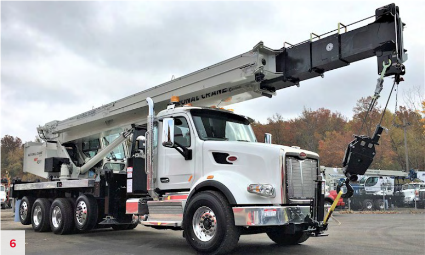
NEW 2022 National NBT45127-1 45 USt, 127' Main Boom, 31'-55' Jib, Wireless ATB, 102" W Aluminum Deck, A/C in Operator's Cab, Single Front Outrigger, and 24" dia. Aluminum Outrigger Pads. Mtd on a Peterbilt 567 Chassis, X-15/ 500 HP, 18-Speed UltraShift Plus-Trans, 20K FA w/Disc Brakes, 46K RA w/Disc Brakes, (2) 13,500 lbs. Lift Axles, Zinc-Coated Anti Corrosion Treated Frame Rails, 100 Gallon Fuel Tank with Heater, Work Lights, and MUCH MORE. EXW Richfield, OH. (Not as pictured) 2 Units in Stock. Unit #R2232.
