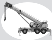
The GRT9165 is designed with a class-leading 205-foot main boom, new wider full vision cab, intuitive Crane Control System (CCS), reduced transport height, and best-in-class load charts.
