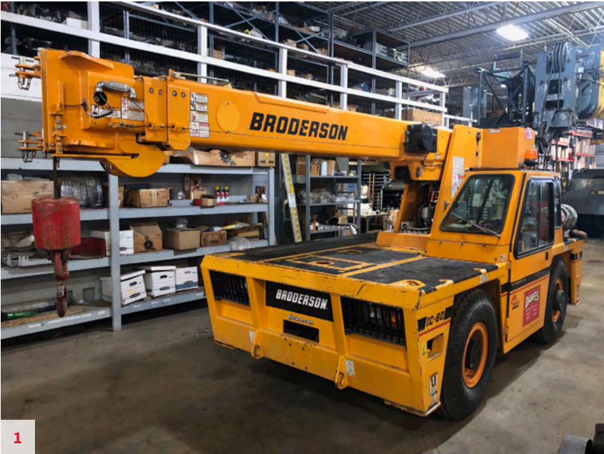
Broderick IC-80-3J, S/N 72214780 2018, 9 USt, GM 3.0 Dual Fuel, 1,200 Hours, 30' Main Boom, 10' Jib, Hoist Drum Rotation Indicators, 4 Wheel Steer, 2 Wheel Drive, Rearview Mirrors, All Weather Cab, Strobe Light, RCL – Greer. Located in Toledo, OH. Unit #11263. $110,000
