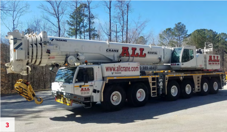
Tadano ATF400G-6, S/N 2063162 2015, 450 USt, Mercedes Diesels, (3,200 Upper Hours), 30,000 Miles, 197' Main Boom, 257' Luffing Jib, 12x8x12 Drive/Steer, 20.5 R25 Tires, Battery Recharge and Remote Start Connection, Air and Electrical Lines for Rear Bumper for Dolly, Boom Removal System, Outrigger removal system (front and rear), ABS. Located in Atlanta, GA. Unit #11055. $2,425,000
