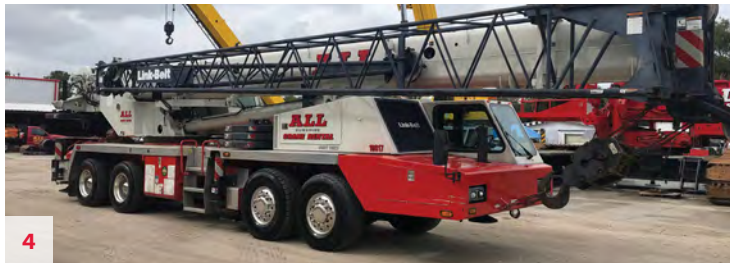
Link-Belt HTC8675 II, S/N P9K3-3595 2013, 75 USt, Cummins ISX11.9, 9,000 Hours, 70,000 Miles, 127' Main Boom, 38'-64' Bifold Jib, Aux. Hoist, A/C in Upper and Lower Cabs, Daytime Running Lights, Amber Strobe Light, Boom Flood Lights, RCL Bar, Trailer Air and Electric, Boom Float Kit, Block and ball. Located in Orlando, FL. Unit #10817. $475,000.00
