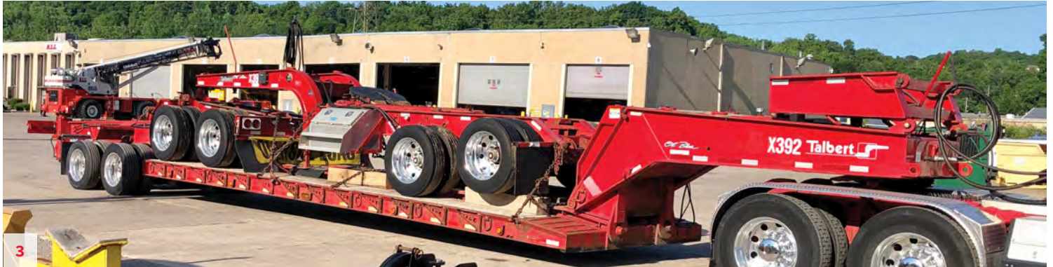
Talbert S/N 40fak2840l1008286 1989, 60 USt 2+2+2 Multi Axle Model T4dw-60-Ra-T1-St 2/2, Turner Air Suspension, Talbert Telescopic Drop Legs, Tool Boxes, Right Weigh Load Scales, Aluminum Wheels, Length 73' 5", Width 9' 3/4", 28' Well, 27' 5" Clear, Empty Weight 50,000, Well Maintained Trailer. Located in Cleveland, OH. Unit #X392. POR
