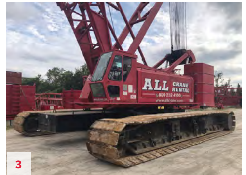
Manitowoc 888, S/N 8881093 1997, 230 USt, Rebuilt Cummins MTA11-C330 (5,335 Hours), 180' Main Boom, Series 2 Counterweights, Self Erect, Ringer Prepped, Hydraulic Powered Crawler Extend/Retract System, LMI. Located in Orlando, FL. Unit #8299. $509,000
