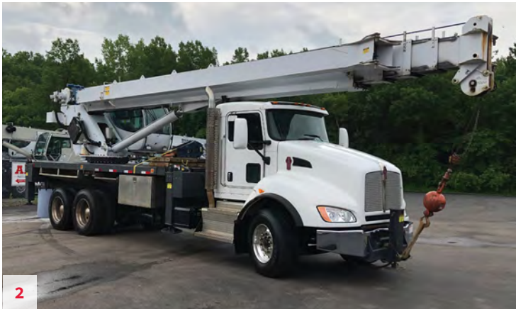
Manitex 40124S 2013, 40 USt, 124' Main Boom, 31'-55' Jib, Steel Bed, Single Front Stabilizer, No Free Swing, Heat and A/C in Operator's Cab. NEW ANNUAL & DOT Inspections. Mtd on a Kenworth T440, Cummins ISL 370HP, Allison Automatic Transmission, 90 Gallon Fuel Tank, and 66,000 GVWR. EXW Richfield, OH. Unit #U2175
