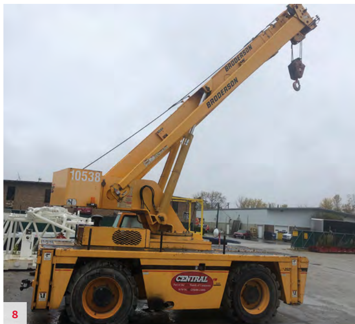
Brodersen IC-250-3C, S/N 35650250 2012, 18 USt, Cummins Diesel (4,700 Hours), Catalytic Converter, Engine Heater, 60'7" Tip Height, 20' Jib, Drum Rotation Indicators, 4 Wheel Steer and 2 Wheel Drive, Headlight and Taillight Grilles, All Weather Cab, Strobe Light, RCL Greer. Located in Chicago, IL. Unit #10538. $129,000
