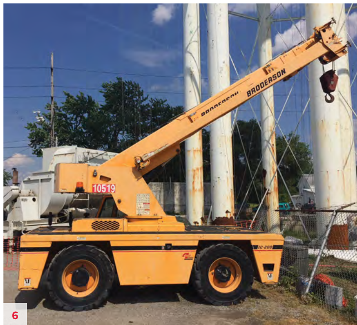
Brodersen IC-200-3G, S/N 222373200 2012, GM Dual Fuel (3,250 Hours), 50' Main Boom, 16' Jib, 2 Wheel Drive and 4 Wheel Steer, Engine Heater, Headlight and Taillight Grilles, Enclosed Cab, Strobe Light, All Weather Cab, RCL Greer. Located in Indianapolis, IN. Unit #10519. $90,000
