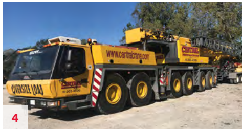
Grove GMK6250L, S/N 6220-9168 2011, 250 USt, Mercedes Diesels, 8,500 Upper Hours, 95,000 KM, 236' Main Boom, 124' Jib, Aux Hoist, A/C in Upper and Lower, Trailing Boom Float Kit, Boom Removal Kit, Hydr. Quick Disconnect for Outrigger Beams, Removable Rear Outrigger Boxes, 20.5R25 Tires, Worklights, Block and Ball, 2 Axle Boom Dolly. Located in Fort Wayne, IN. Unit #10464. $995,000
