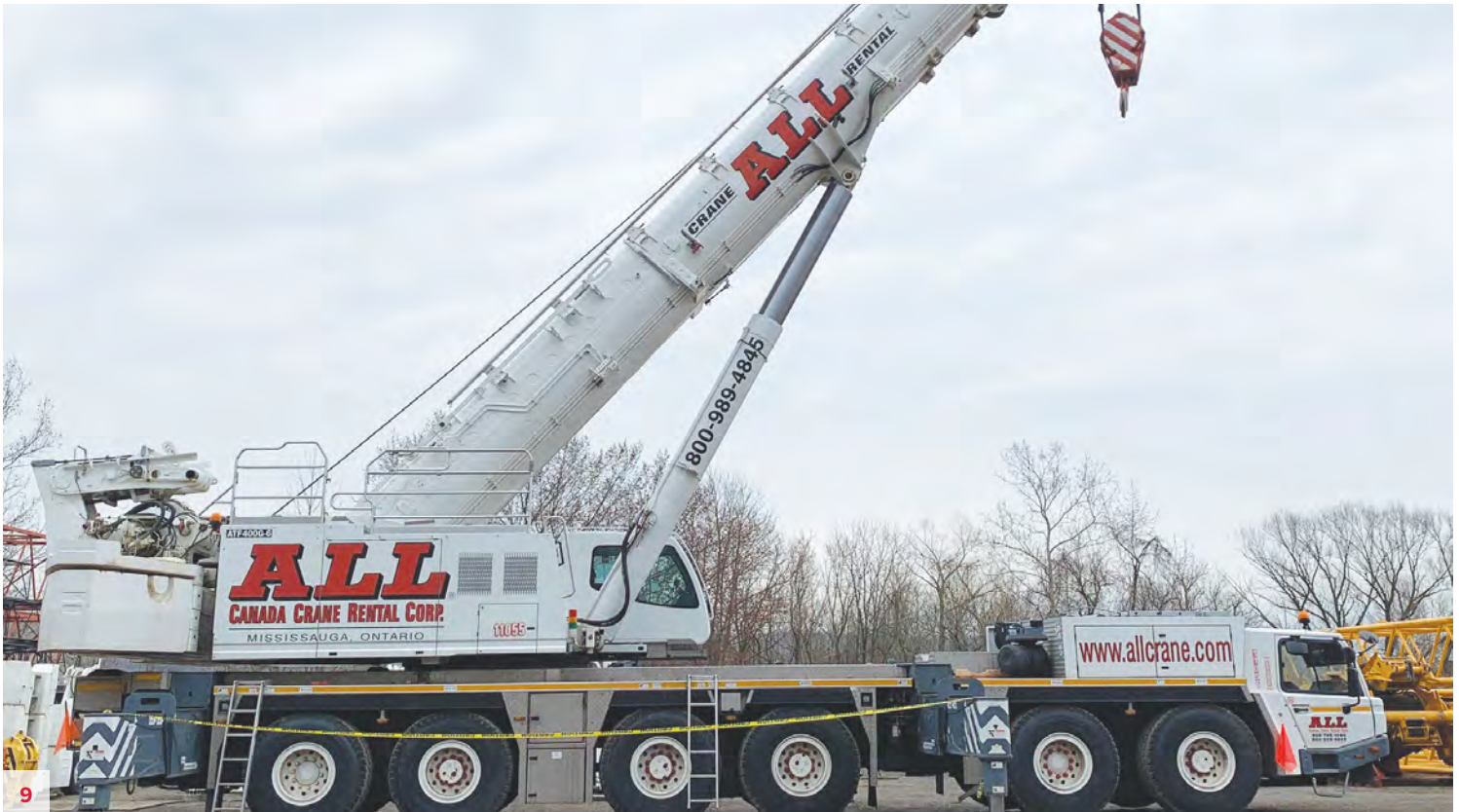
Tadano ATF400G-6, S/N 2063162 2015, 450 USt, Mercedes Diesels, 3,100 Upper Hours, 24,500 KM, 197' Main Boom, 257' Luffing Jib, 12x8x12 Drive/Steer, 20.5R25 Tires, 2 Working Lights on Boom, Battery Recharge and Remote Start Connection, Air and electrical lines for rear bumper for dolly, Boom Removal System, Outrigger removal system (front and rear), Additional independent heater with engine, ABS. Located in Atlanta, GA. Unit #11055. $2,750,000
