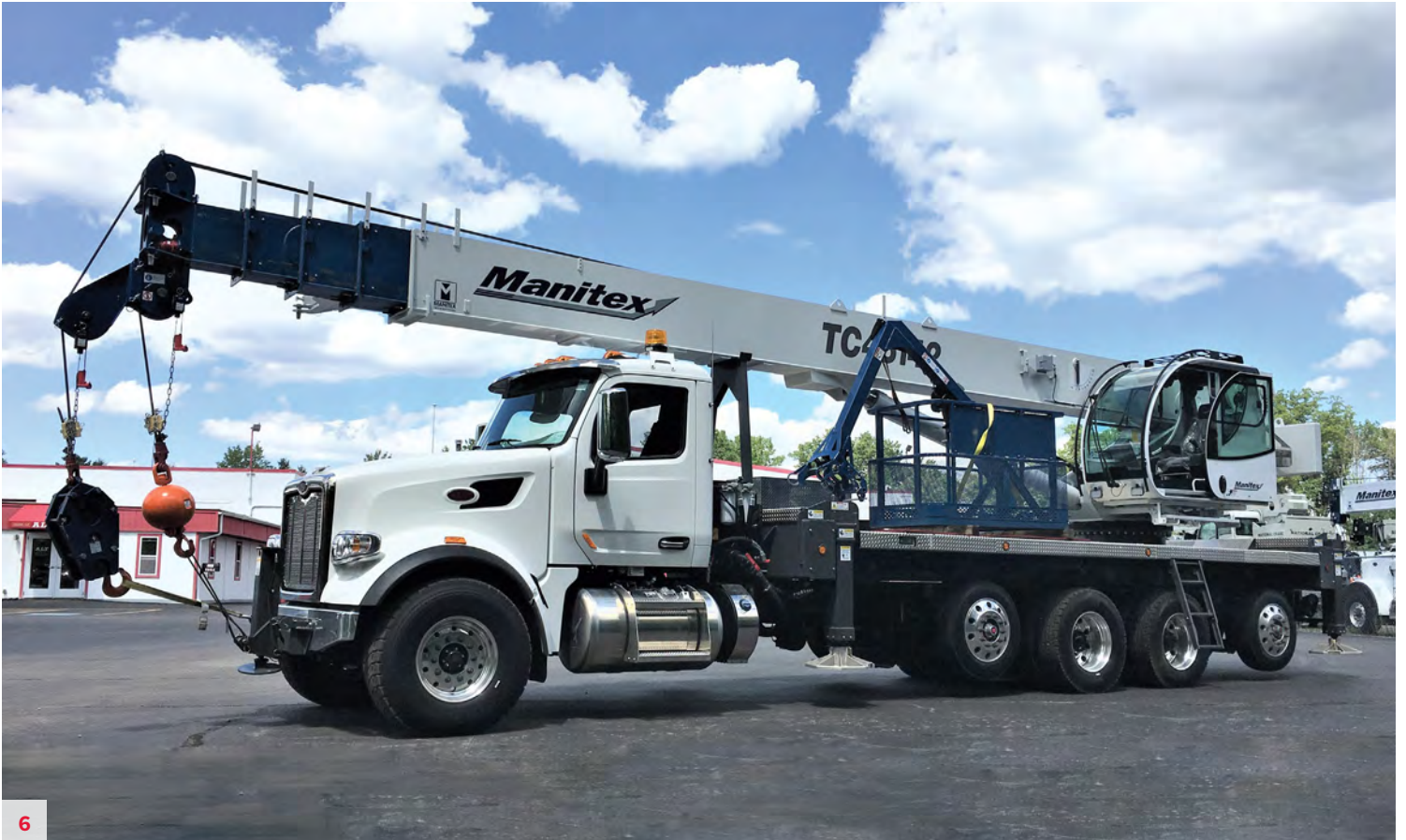
NEW Manitex TC45142 45 USt, 142' Main Boom, 31'-55' Jib, 18 Month Warranty, Remotes, A92.2 Rated (Removes need for test weights) 2 Man LW Basket, 2 Braden Winches, and MUCH MORE. Mtd on a Peterbilt 567, X15 500HP, 13-Speed UltraShift Transmission, 20K FA, 13,500 Pusher, 46K Tandem 13,500 Tag, 100 Gallon Fuel Tank. EXW Richfield, OH. Unit #R2152
