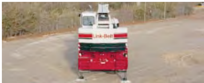
Retracted Outriggers 7' 9" (2.36 m) Spread
