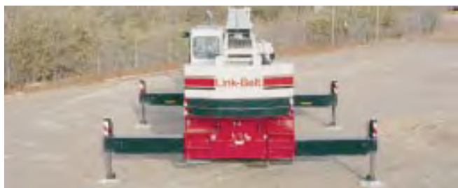
Fully Extended Outriggers 20' 6" (6.25 m) Spread
